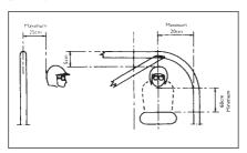
**16.4.** The upper part of the driver and co-drivers helmet must be at least 5 cm below the top of the rollbar hoop. Ref. Drawing Appendix 6.
